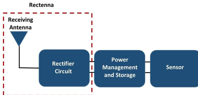
Fig. 1: components of an RF harvesting system
