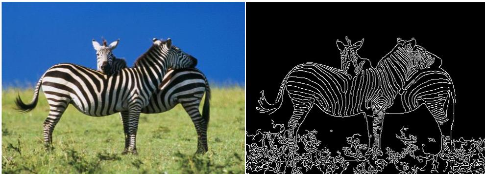
**Fig. 1.** Original image on the left and edge detection on the right.
