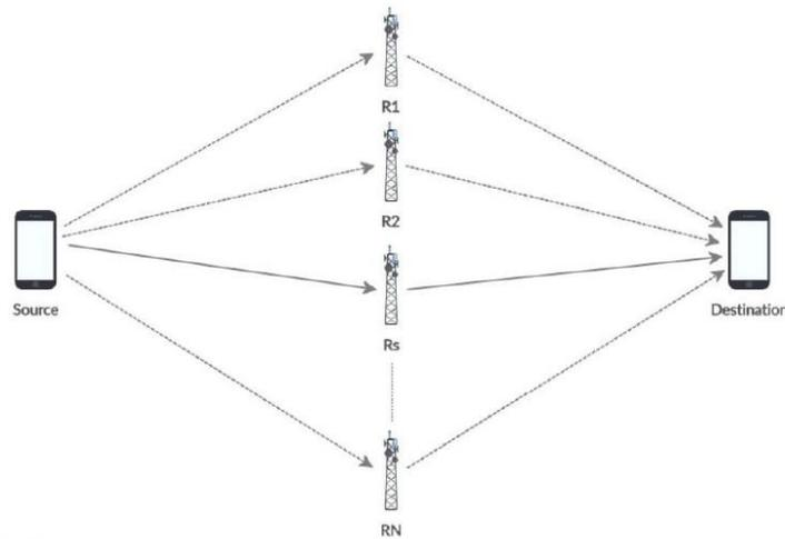
**Fig. 3.** A hybrid AF/DF relaying network which selects a single relay out of  $N$  available ones.
