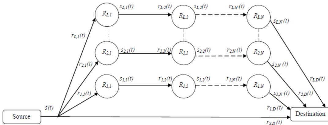
**Fig. 2.** A hybrid AF/DF multi-hop multi-branch relaying network.
