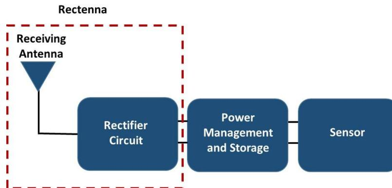
Fig. 1: Block Diagram of a rectenna system
